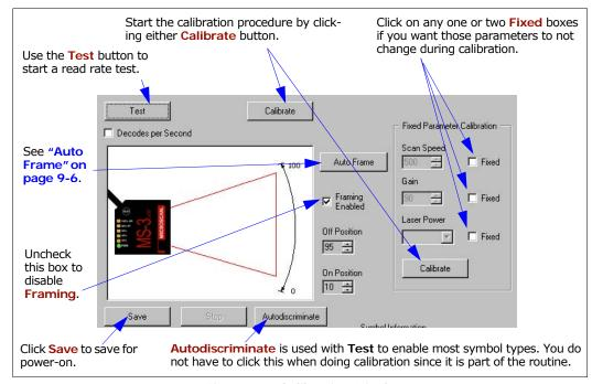
Figure 9-7 Calibration Display
