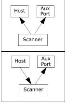
Serial Cmd: < K101,aux port mode, baud rate, parity, stop bits, data bits, daisy chain ID status, daisy chain ID>
