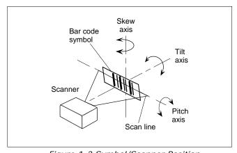
Figure 1-3 Symbol/Scanner Position
