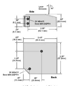
MS-3 Integral Right Angle Laser Scanner
