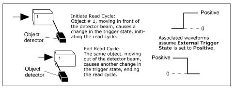
Figure 4-2 External Level Trigger
