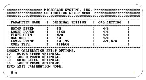
Figure 9-8 Embedded Calibration Setup Menu
