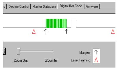
green waveform indicates a decoded symbol; a red waveform indicates an undecoded symbol or other object.
